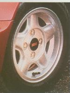
Giving an edge to that legendary handling, the Cabriolet is fitted with 5-spoke Revolution alloy wheels with 165/60 X 12 low profile tyres
