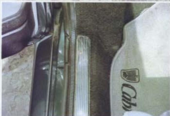
When you remove the roof of a monocoque, the floorpan has to be strengthened. Here's a beefy sill section for beam stiffness.
