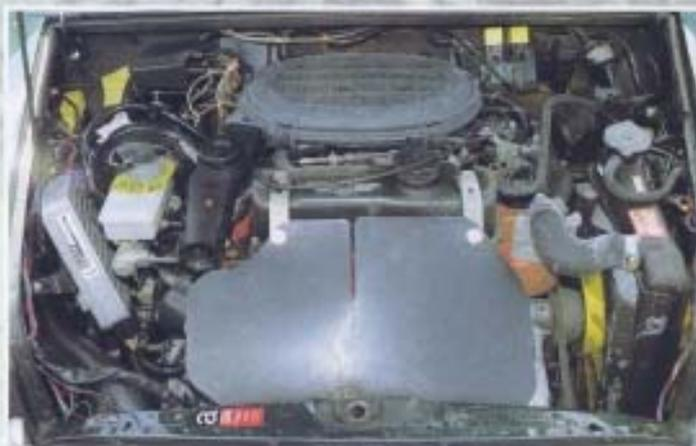
Typical A+ Rover 1275 injection unit with MEM5 ECU and single-point fuel
