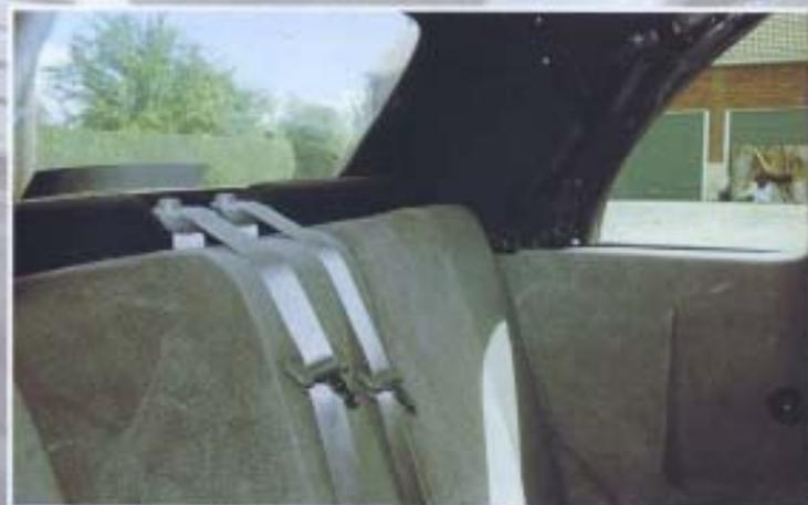
Hood up in the rear, rear belts are inertia with reels mounted centrally.
