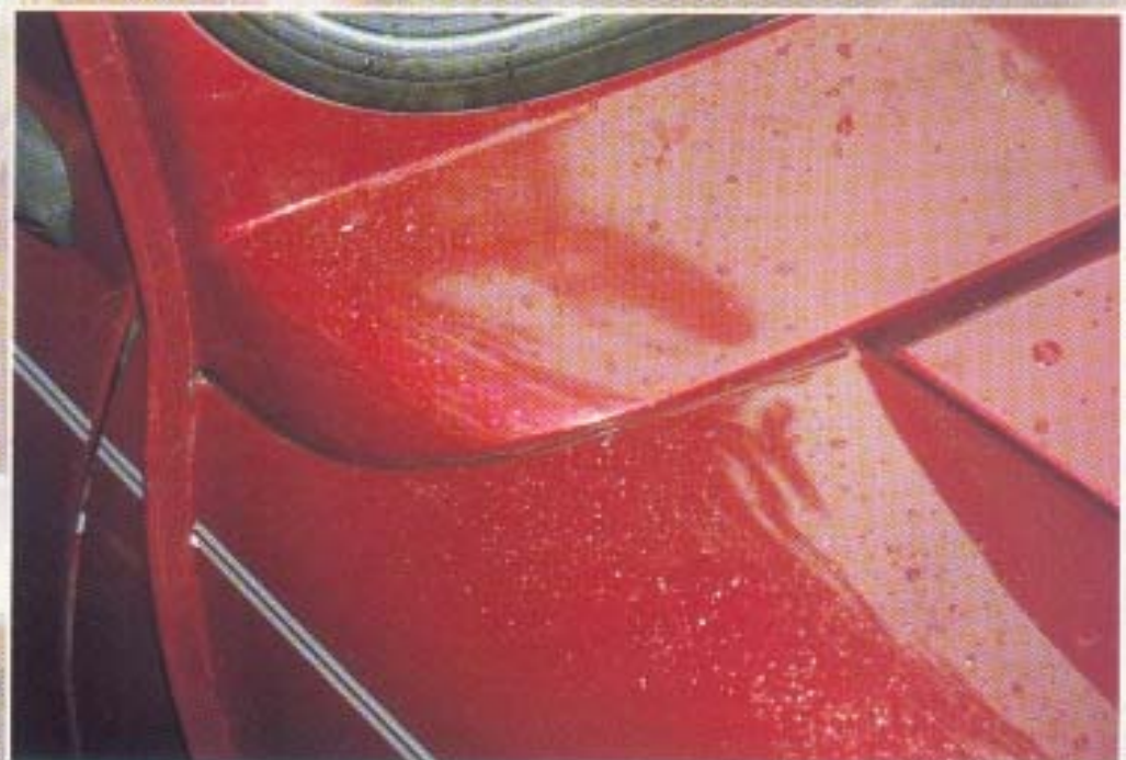
Make the usual checks for rust around the seams. Lamms still mostly too young for bad rust problems.
