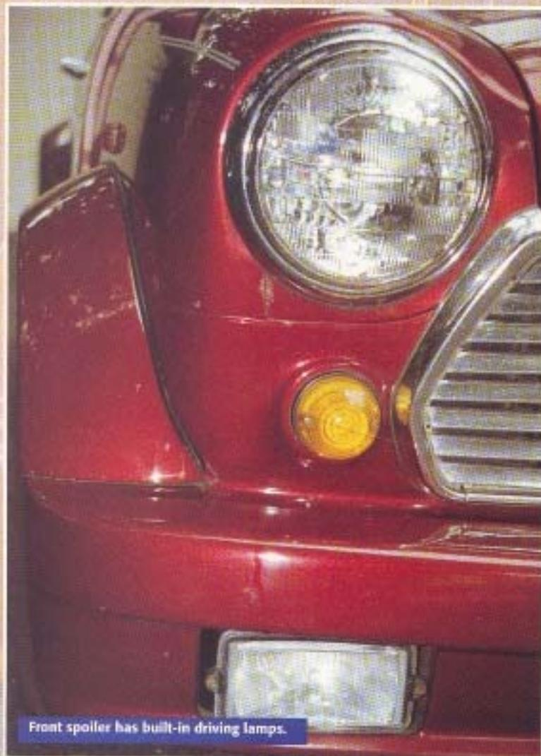
Front spoiler has built-in driving lamps.
