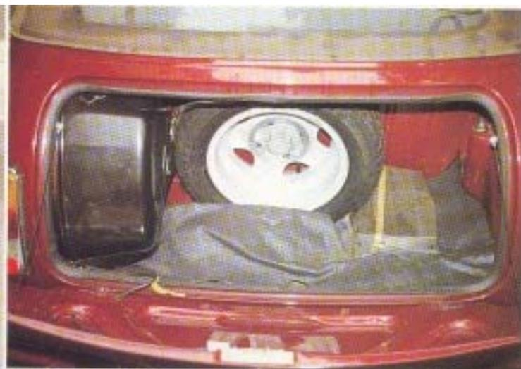
Vertically-mounted spare wheel - doesn't fit into usual spare wheel well.
