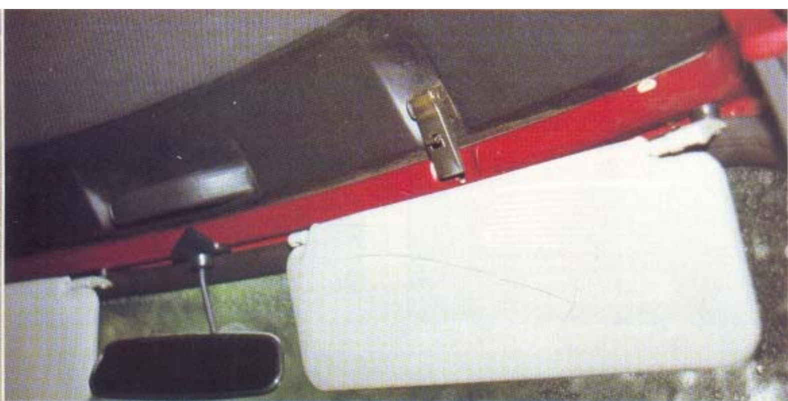
Hood catches are cleverly hidden behind sun visors.
