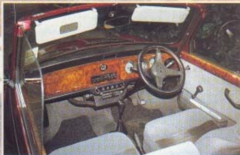
Interior has plenty of wood trim, including door cappings.
